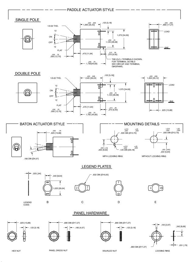
Notes: 1 All dimensions are in inches [millimeters]. 2 Tolerance ±020 [.51] unless otherwise specified.
