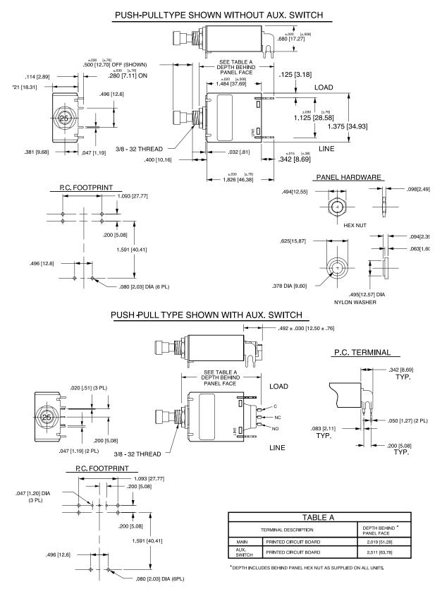
Notes All dimensions are in inches [millimeters]. Tolerance ±.020 [.51] unless otherwise specified. 1 2
